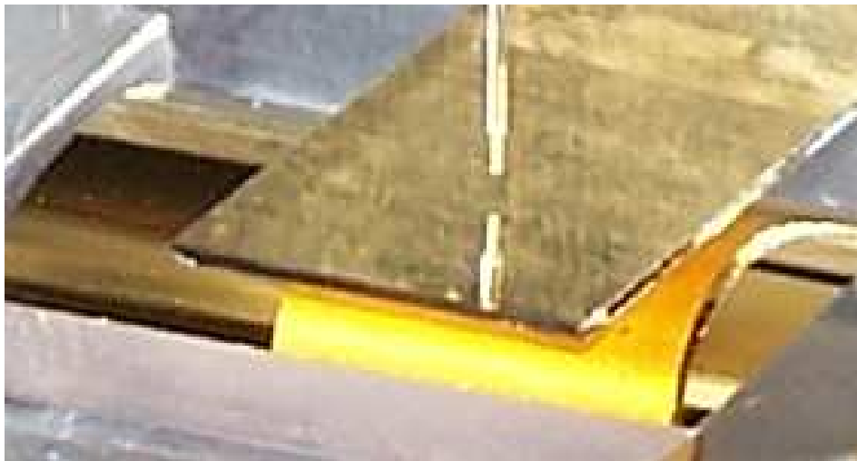
FIG. 4: Image of the experimental set-up for the study of the cylinder-plane configuration, with (from top to bottom) the optical fiber for the displacement measurement, the silicon rectangular cantilever, and the cylindrical lens. Cantilever and cylindrical lens, coated with (144 \pm 20) nm of Au, have respectively width and radius of curvature equal to 1 cm. Notice the mirror image of the optical fiber on the cantilever, which allows to estimate the fiber to cantilever distance. With proper illumination and the use of an optical microscope by looking at the mirror image of the cylinder on the cantilever, it is likewise possible to estimate the cylinder-cantilever distance at large (above \simeq 10 \mu\text{m} ) gaps, which allows for consistency checks with the electrostatic calibrations.
